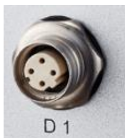
Fast Ethernet - M12 D-Code 4-PIN, Female
